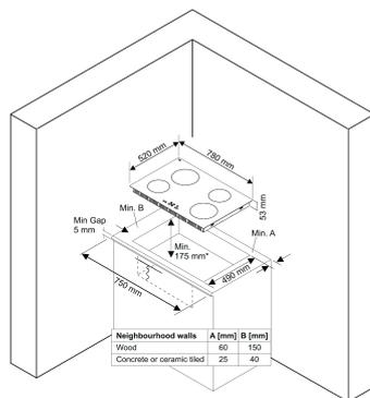
\* In the case of installation over built in oven, distance should be min. 10 mm.
